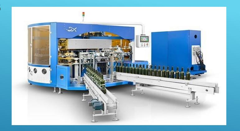
Fully automatic turntable machine 6 color screen printing 1 hot stamping QR code detection
